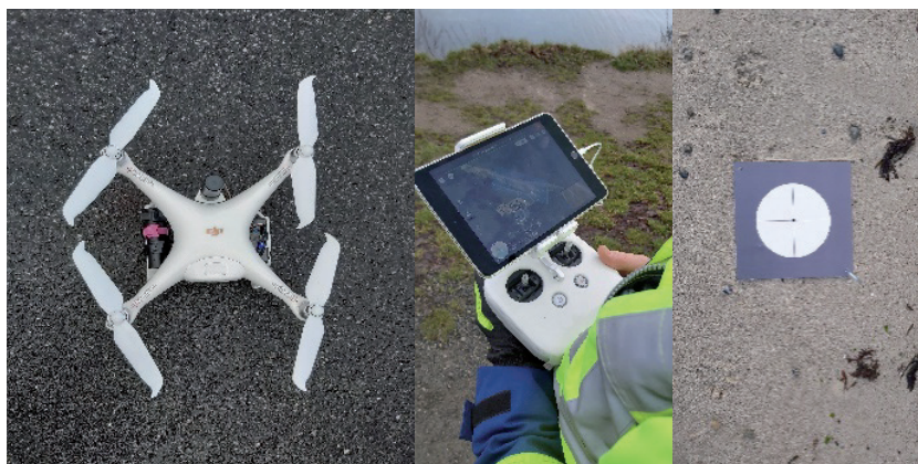
Fig. 3: DJI Phantom 4 Pro KlauPPK (left), remote control with Apple iPad (centre) and signalised ground control point (right)
