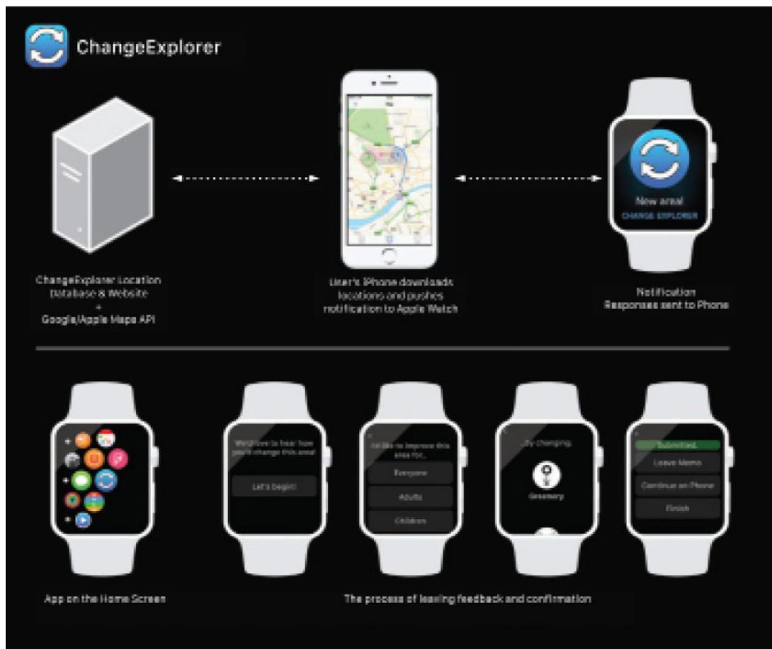
Figure 27: Details of ChangeExplorer's client server architecture and screen shots of the watch's interface: screen shots of the notification being received, the app on home screen, and the process of leaving feedback and confirmation
