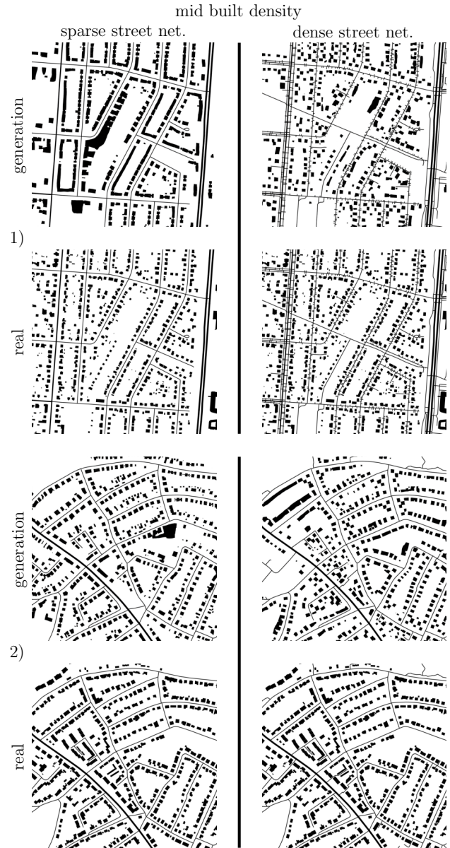
Figure 6. Comparison of two generated figure-ground maps with a mid built density trained with sparse (left) and dense (right) street network data with a spatial resolution of 1:8000.
