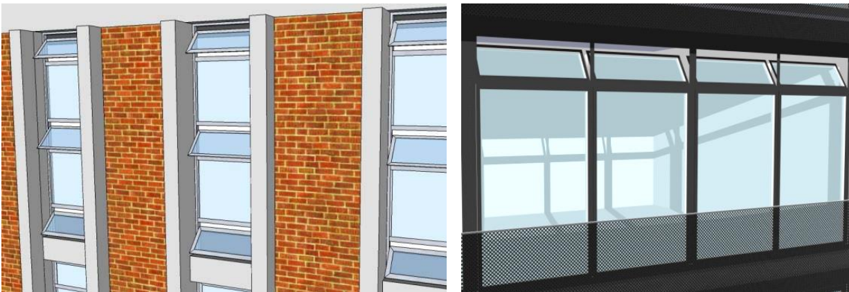
Fig. 4: Illustration of the openings for ventilation of IFCH Campinas (left) and HafenCity University, Hamburg (right)
