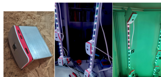
Figure 3. Raspberry Pi camera with the mounting bracket (left), low-shadow lighting due to LED strips (centre), coloured lighting to indicate system status (right).
