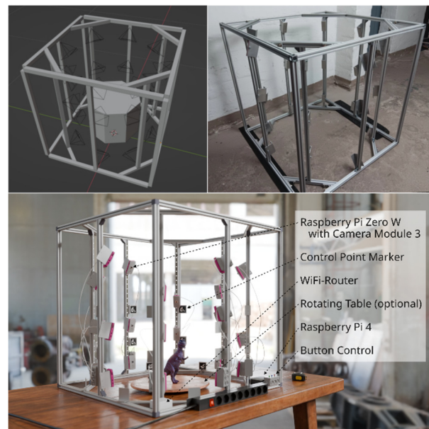
Figure 2. Design of the photogrammetric low-cost 3D measurement system (top left) and realised aluminium frame (top right). Setup of the photogrammetric low-cost 3D measurement system using 24 Raspberry Pi cameras (bottom).
