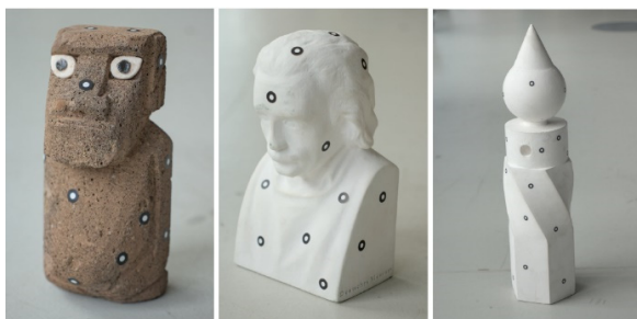
Figure 1. Reference objects (Moai figure, Einstein bust, and Testy) for testing the multiple Raspberry Pi cameras setup.
