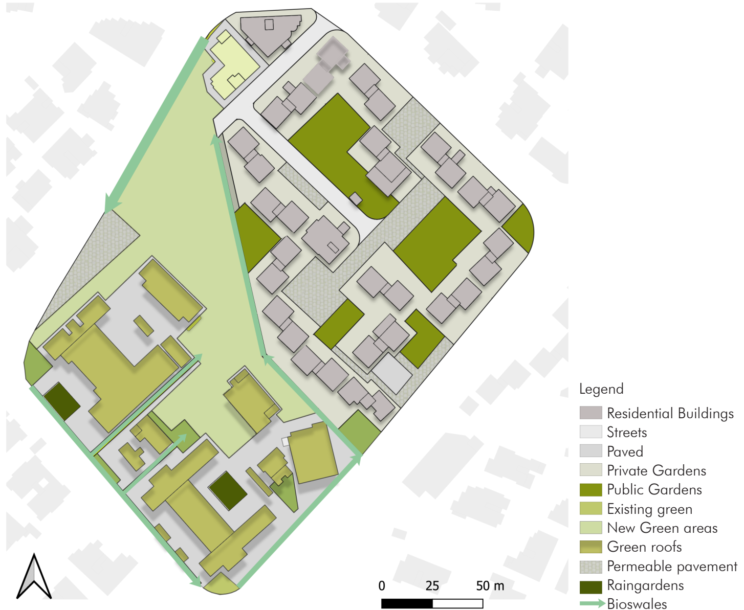
Figure 59: Map of Scenario 2 - Conceptual design of measures in public areas Source: Author
