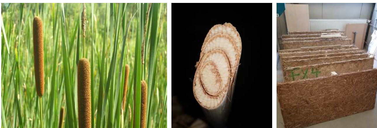
Figure 3: Typha plant; Leaf bundle cross-section; Load-bearing and insulating magnesite-bonded Typha board. Image Source: Left – Petr Filippov, Wikimedia Commons; middle – Fraunhofer IBP; right – Fraunhofer IBP.
