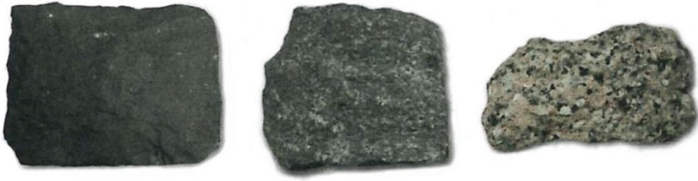
Figure 2.4: Extrusive and intrusive igneous type of rocks. From left to right: basalt, gabbro, and granite (Grotzinger and Jordan, 2020).
