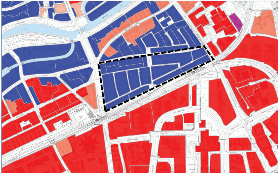
Figure1: Preliminary target scenario for the heat supply of the “Gartenstadt Alsterdorf” neighbourhood (map excerpt from the Hamburg Heat Register; scale 1:5,000; accessed 17 March 2026). Blue: decentralized heat supply; red: existing district heating networks; light red/beige: district heating expansion likely; pink: decentralized and district heating both possible; black dotted area: study area.
