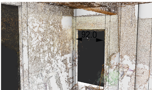
Fig. 3.5.1: reference measurement overlay pointcloud and 3D Model
