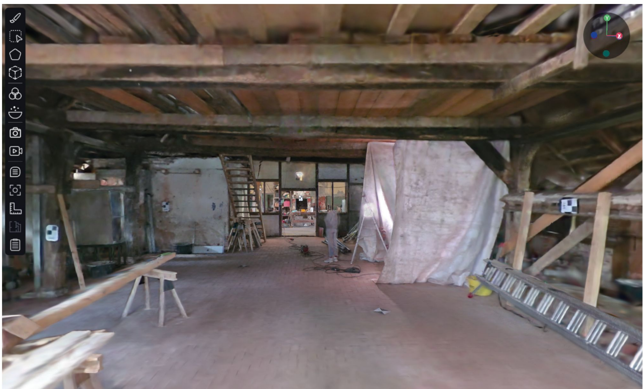
Fig. 2.5.1: Gaussian Splat of the mainroom created with LCC Studio
