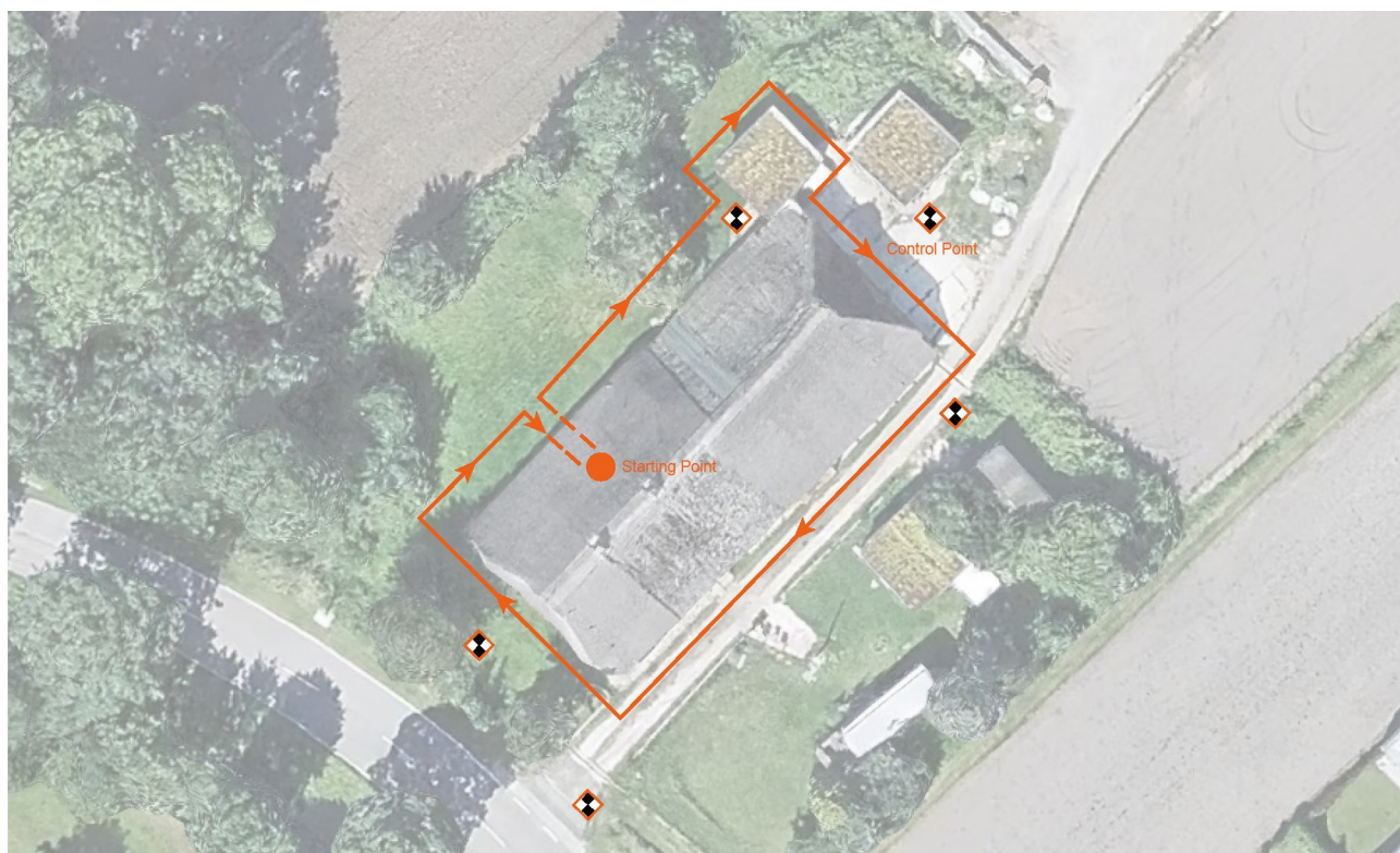
Fig. 2.3.3: Areal view of the Hufnerhaus with control points and scanning route
