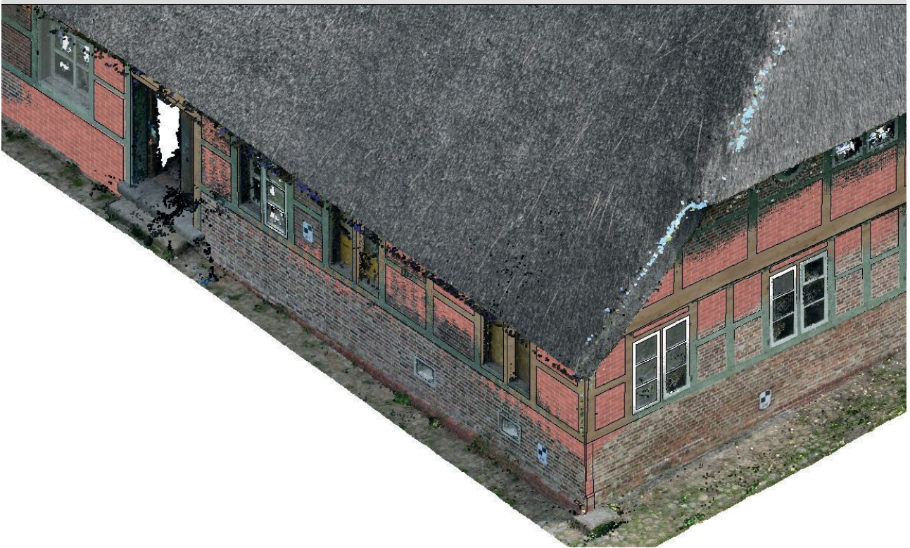
Fig. 1.4.11: Overlay of the point cloud and the BIM model front
