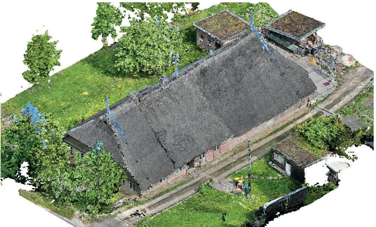
Fig. 1.4.7: 3D point cloud from Agisoft Metashape in Archicad
