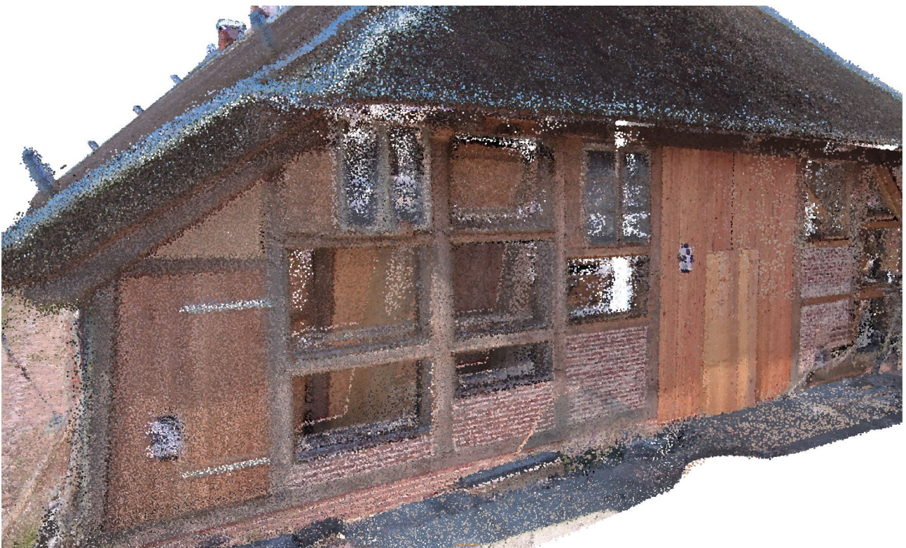
Fig. 2.5.5: Point cloud of the northern facade of the Hufnerhaus in Archicad
