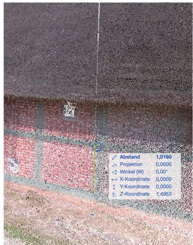
Fig. 2.5.3: Measurement in the point cloud in Archicad
