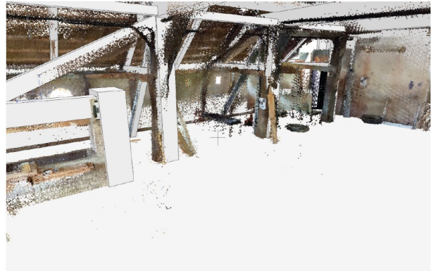
Fig. 5.4.9: Blending the point cloud with the CAD model
