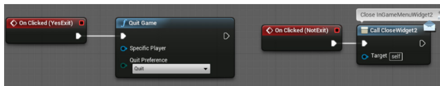
Figure 9-48: Widget “InGameMenuWidget2”: Once the button to quit the game has been pressed, the function “Quit Game” is called to end the application
