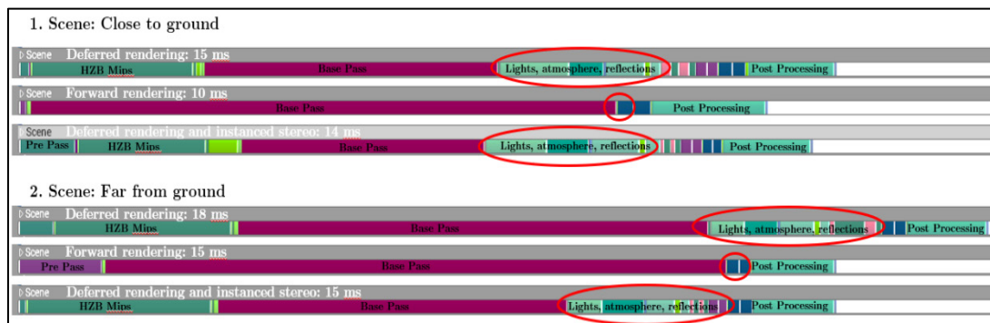
Figure 6-3: GPU cost of various passes (PrePass, Base Pass, Lights, Post Processing) for two scenes with three different rendering techniques. The first scene is close to the ground whereas the second scene depicts an overview of the entire world. The first rendering method is the deferred technique followed by the forward technique and the combination of deferred and Instanced Stereo technique
