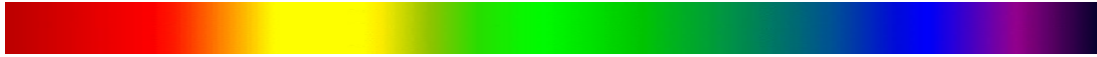
Figure 4-3: Rainbow colour ramp used to colour the terrain corresponding to a given height range.
