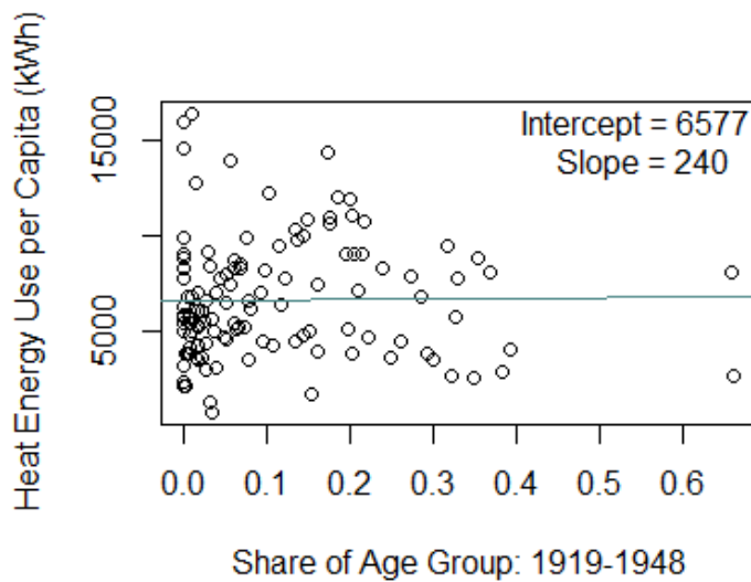
Figure 139: Scatterplot of Heat Energy Use per Capita ( Y_{02} ) and Age Group 2 (1919-1948) ( X_{age2} ) (Author, 2018)
