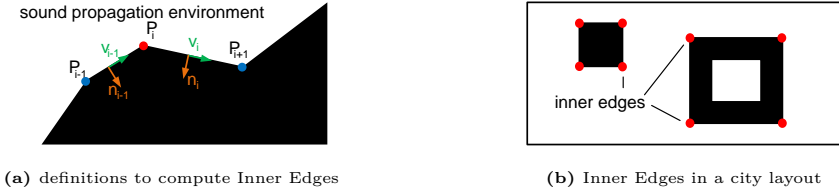
Figure 4.3.: Construction and example of Inner Edges.
