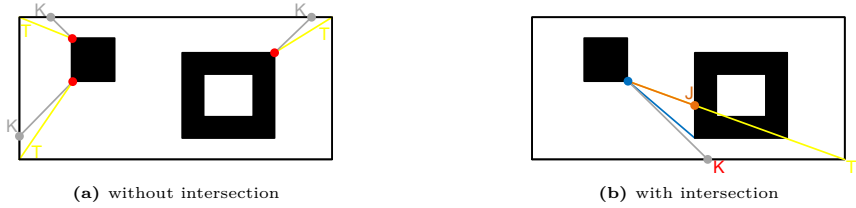
Figure 4.4.: Translation of a Virtual Wall either to the starting point or the end point of the intersected wall.
