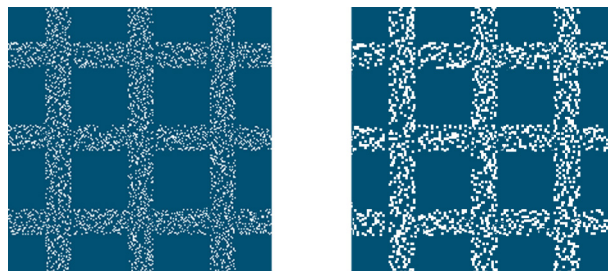
Figure 5.4. Design parameter “noise grain.” Both grids represent the same degree of uncertainty (100%), but with different grain sizes: “fine” (left) and “coarse” (right).
