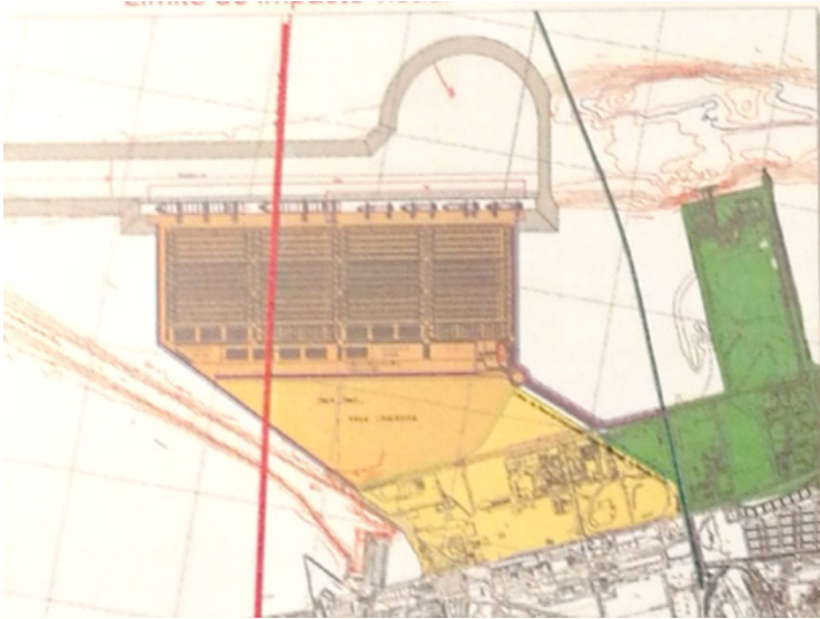
Figure 80 In the image we see the terminal layout proposed by AT Kearney consulting and engineers. The red line was the limit defined by the municipality to protect the view over Lisbon. In the same report we can read that respecting this limit would reduce the terminal from 2,1 to 1,3 million. The first section of the terminal would not compromise the view, but for economic and environmental issues it was recommended to build the landfill in a single stage. Hence it was necessary to decide at the beginning if the terminal would overpass the red line. In the report we could read that AT Kearney advised to follow the most profitable version of the terminal, i.e. the two phases overstepping the red line, but that it would require the conscious choice of going against the boundaries set by the municipality. The red line is also visible in images from Amaral (2015). Image retrieved from internal document available in APL's documentation centre (n.d.)
