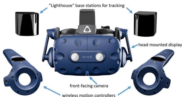
**Fig. 16** The components of the virtual reality system HTC Vive Pro (www.vive.com)
