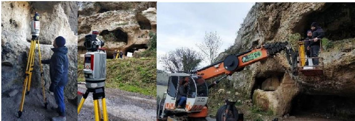
**Fig. 8** Terrestrial laser scanning using the Riegl VZ-400 inside (left), outside the cave (centre) and in hard-to-reach areas using a crane (right)
