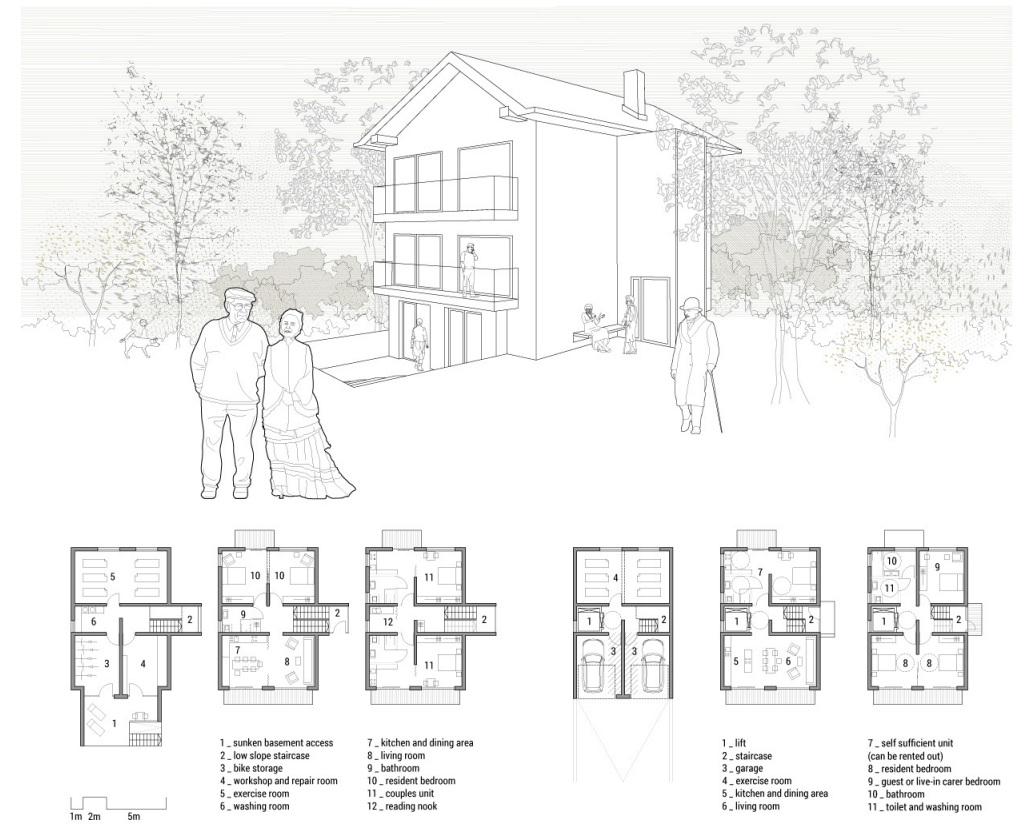
Fig. 3: Two possible floor plan outcomes for the pattern-book house type 2HP-188A, generated using the simplified shape grammar
