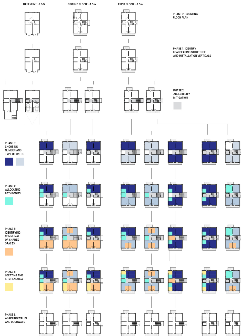
Fig. 2: Example of a simple shape grammar for re-designing the pattern-book house type 2HP-188A into a co-housing unit
