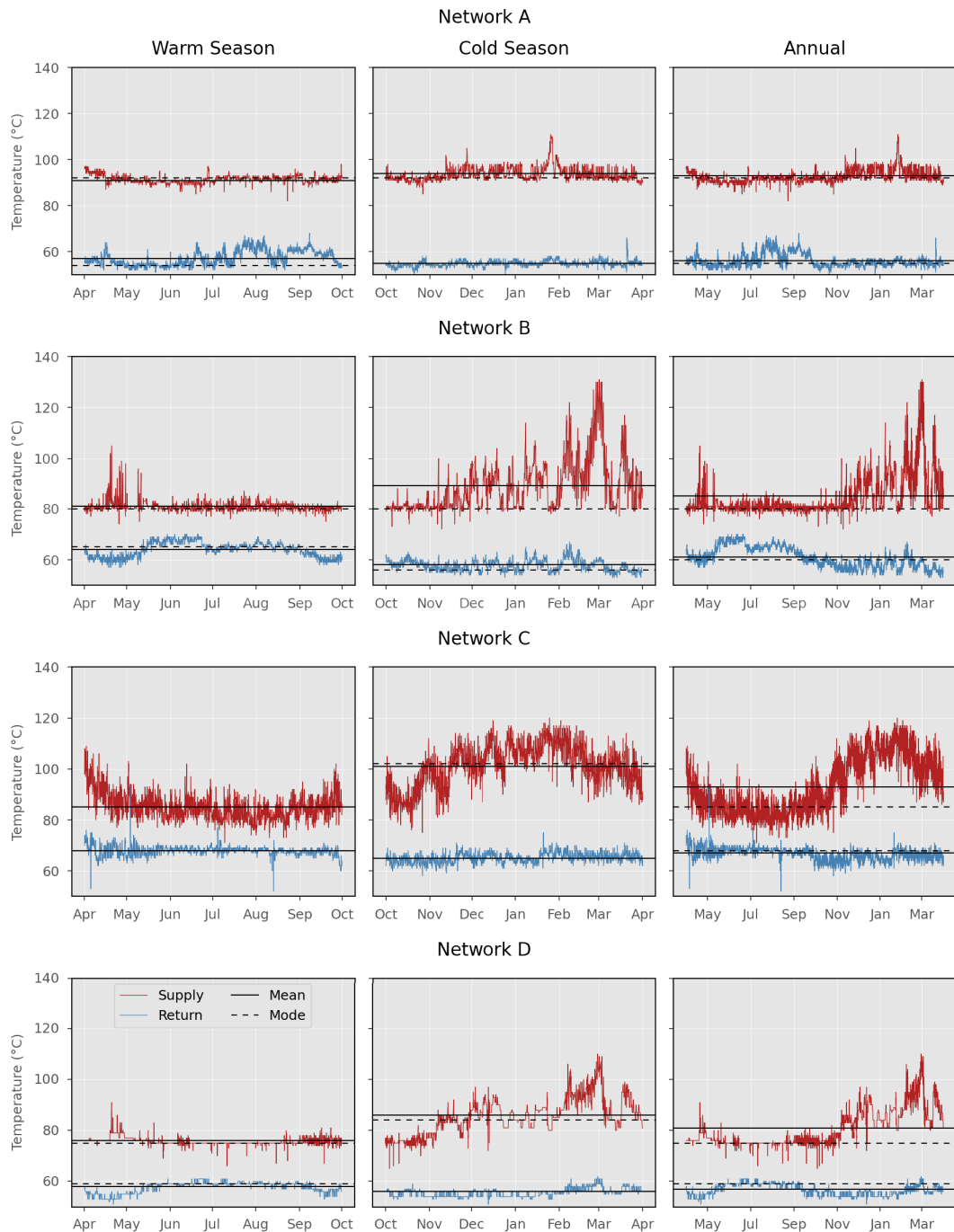
Fig. 2: An annual and seasonal operational temperature pattern of four district heating networks in Germany
