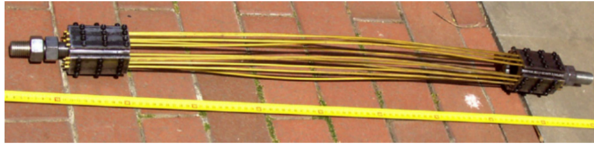
Figure 5. SMA-based damper wires, reprinted from Torra et al. (2007). 1
