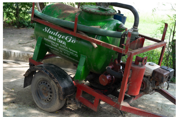
Figure 53 Sludge-Go vacuum tank (source: Author, 2021)
