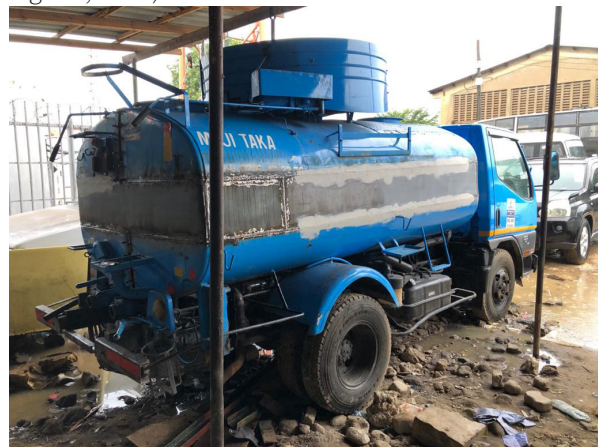
Figure 64 Vacuum truck with expanded capacity (source: Godlove Ngoda, 2019)
