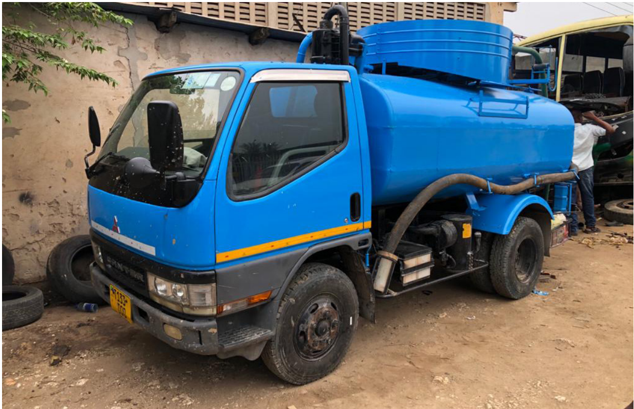
Figure 66 Expanded and repainted vacuum truck (source: Godlove Ngoda, 2019)
