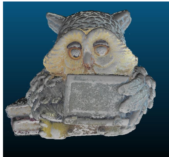
Figure 10: Successful alignment process between reflection and SL point clouds
