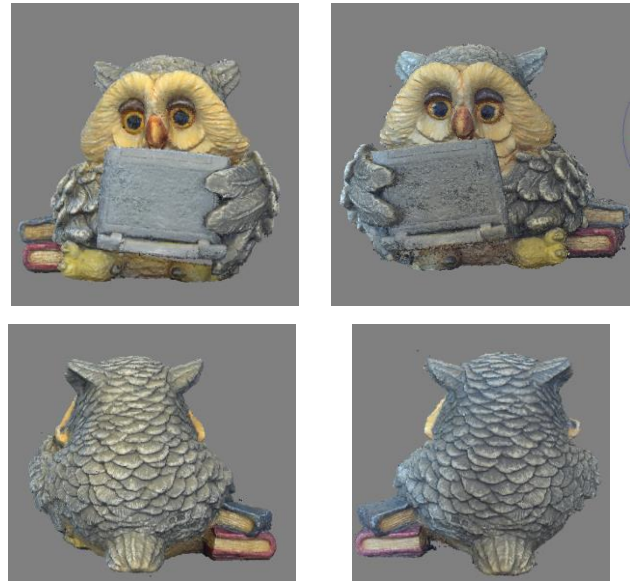
Figure 6: 3D point cloud of both parts of the real object (left) and of its reflection (right)
