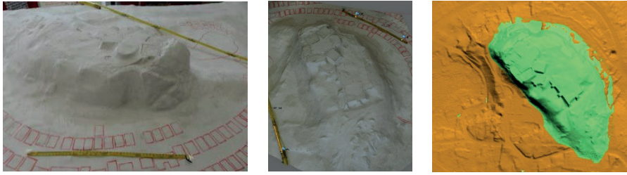
Figure 5. The historic physical 3D model of the Kalkberg (left), the historic digital 3D model from dense image matching (centre) and the combination of two DEMs from both today (orange) and the past (green) (right).
