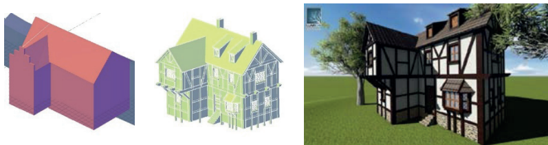
Figure 9. Development of a building in the outer ward: Initial CAD model (left), detailed model (centre), textured model in Lumion 3D (right).
