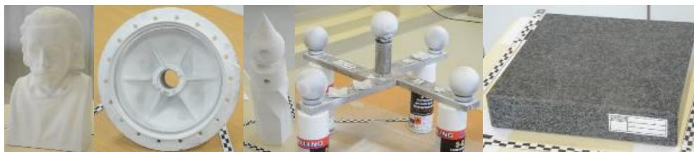
Figure 2. Test and reference bodies for the investigations of the hand-held 3D scanning systems – f.l.t.r. Einstein bust, wheel hub, Testy, cross-shaped body with spheres (centre) und granite slab (right)
