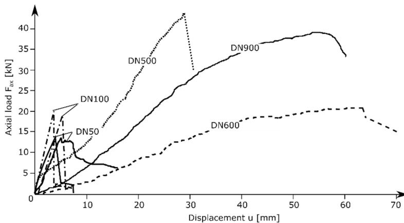
Fig. 3. Examples for shear test results according to EN253 [4].
