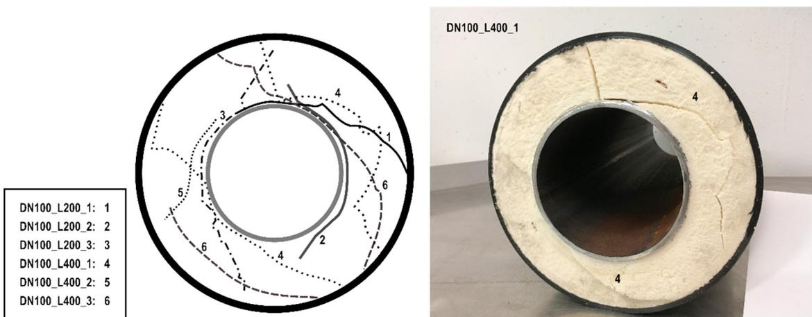
Fig. 5. Observed cracks at the bottom of the samples.
