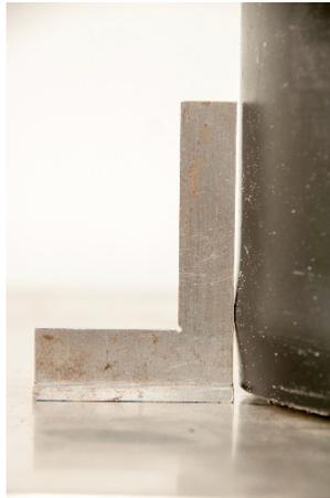
Fig. 6. Local buckling of the coating (DN100\_L400\_2).
