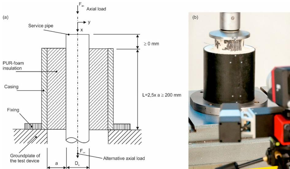
Fig. 1. (a) Test setup scheme; (b) test setup image.
