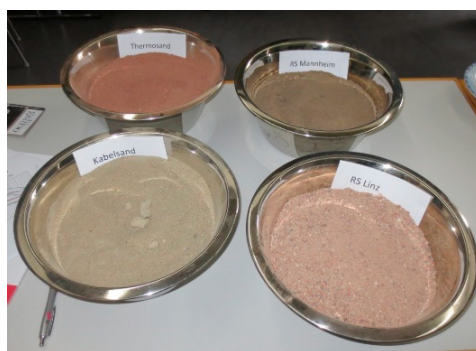
Fig. 4. Recycled material for backfilling in district heating systems.
