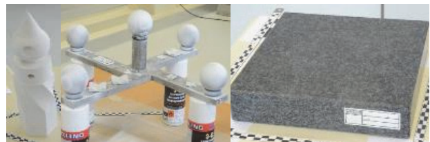
Figure 1. Reference bodies for the investigations of the hand-held scanning systems – Testy (left), cross-shaped body HSBO with spheres (centre) und granite slab (right)
