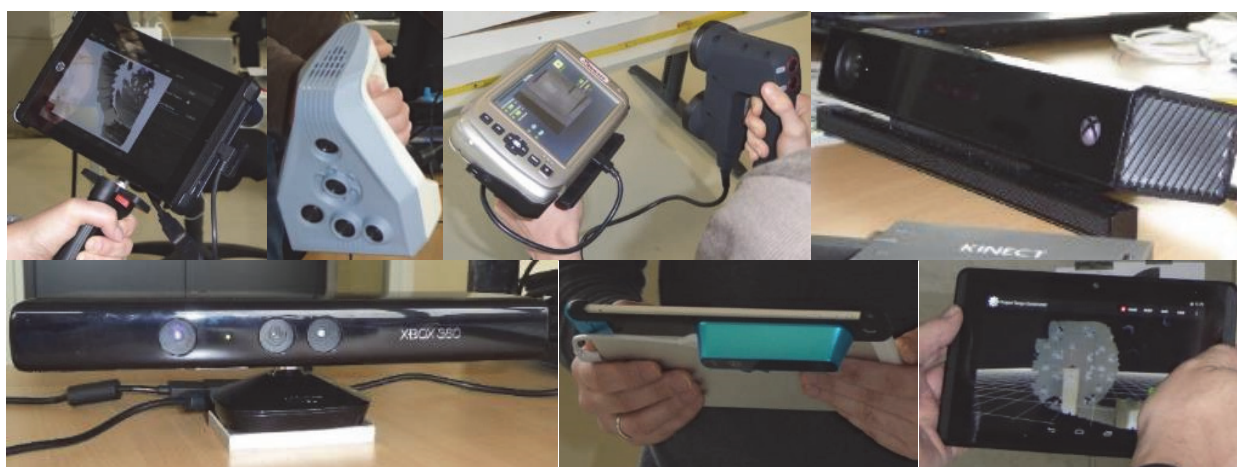
Figure 2. Examined hand-held scanner system (f.l.t.r.) – DPI-7, Artec Spider, Mantis Vision F5, Kinect v2 (top), Kinect v1, Structure Sensor and Google Tango (bottom)
