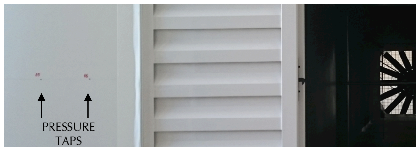
Figure 5. Board with a window sample and pressure taps on the left.
