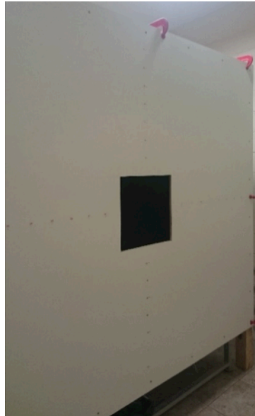
Figure 3. Board fixed at the inlet of the wind-tunnel with an orifice of 40 x 40 cm.
