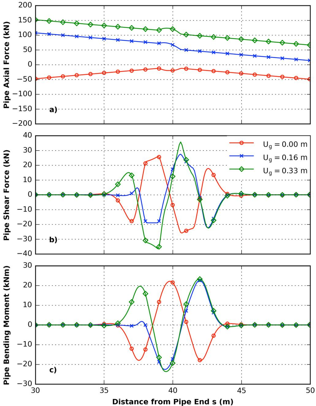
Fig. 3 Variation of the loads along the pipeline axis for different values of the ground displacement  $U_g$ : a) axial force; b) shear force; c) bending moment.
