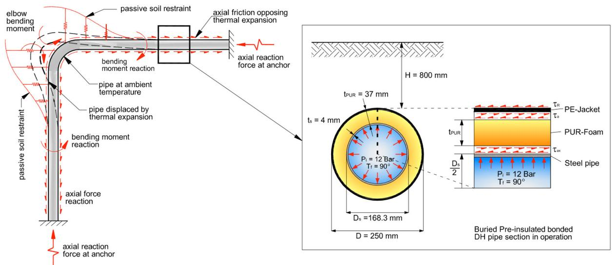
Fig. 1. Deformation of buried operating DH pipeline at the bend (adapted from [4] and [5])
