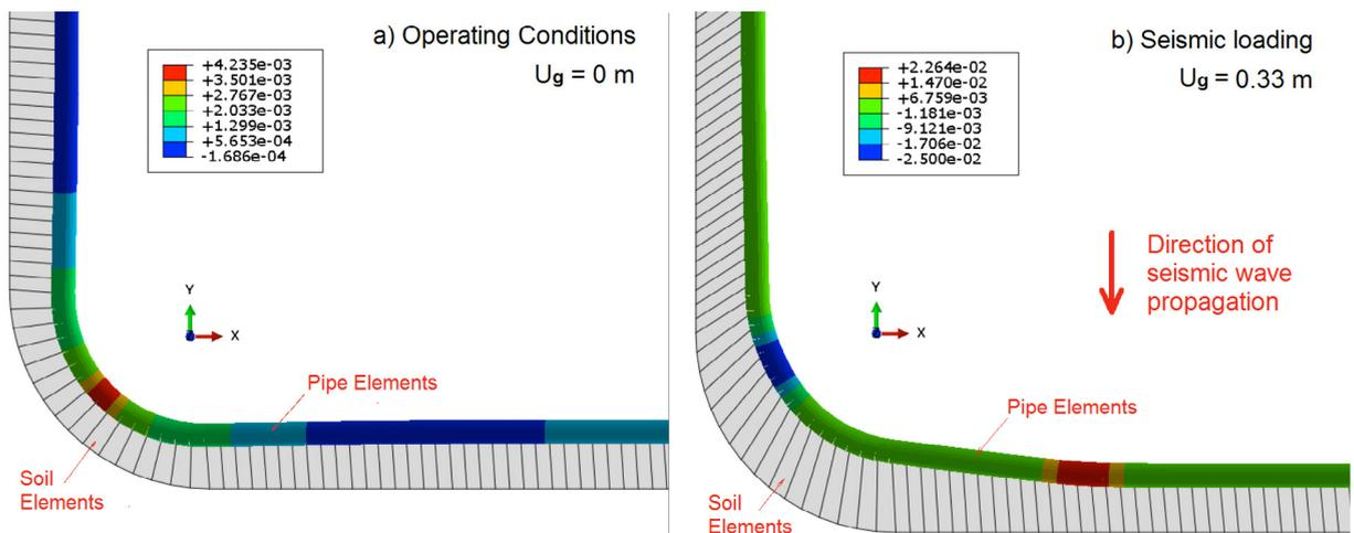
Fig. 6 Longitudinal strain contour and deformed shape of the pipeline at the bend region: a) in operating conditions; b) under seismic loading.
