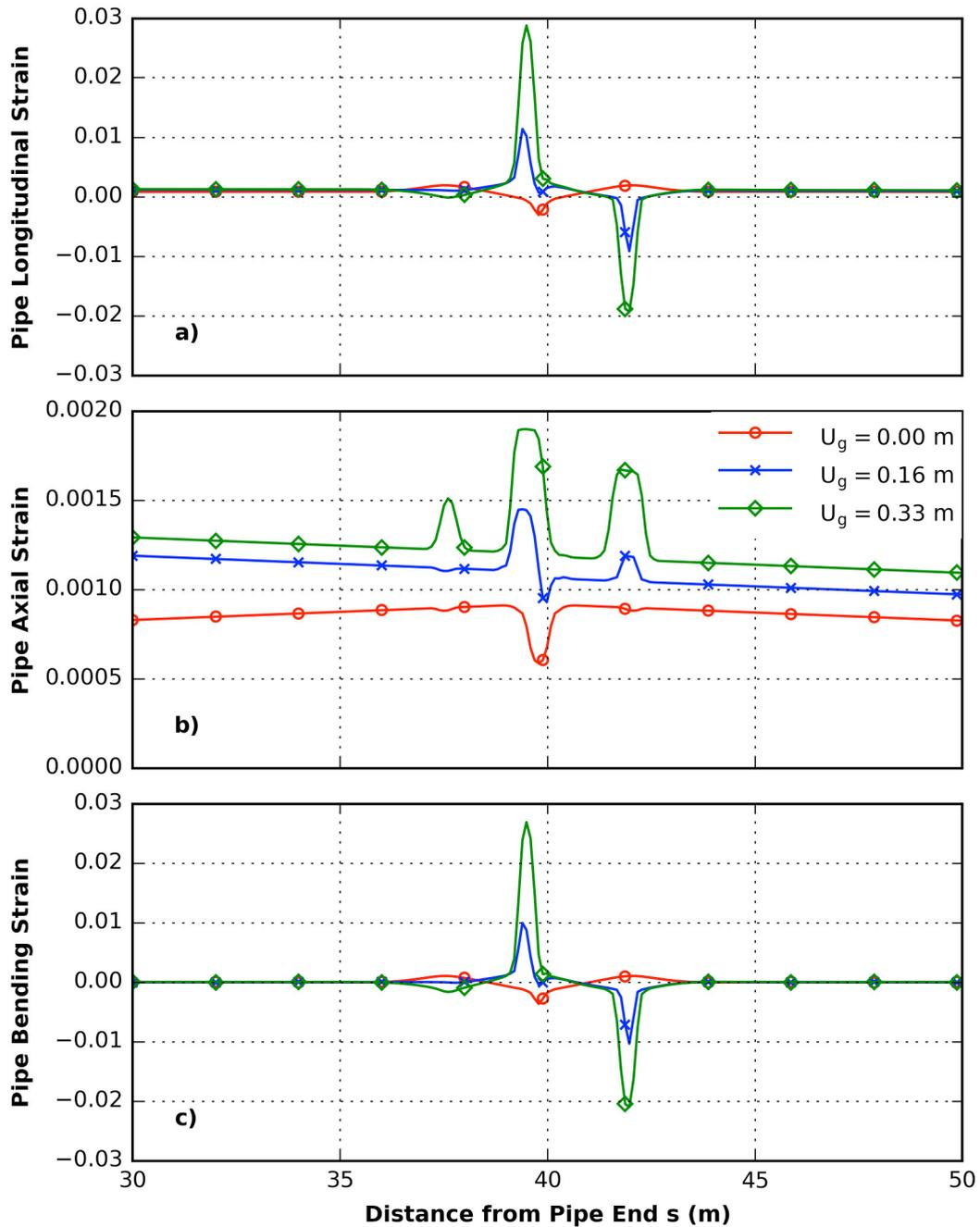
Fig. 4 Variation of the strains along the most stressed generator of the pipeline for different values of the ground displacement  $U_g$ : a) longitudinal strain; b) axial strain; c) bending strain.
