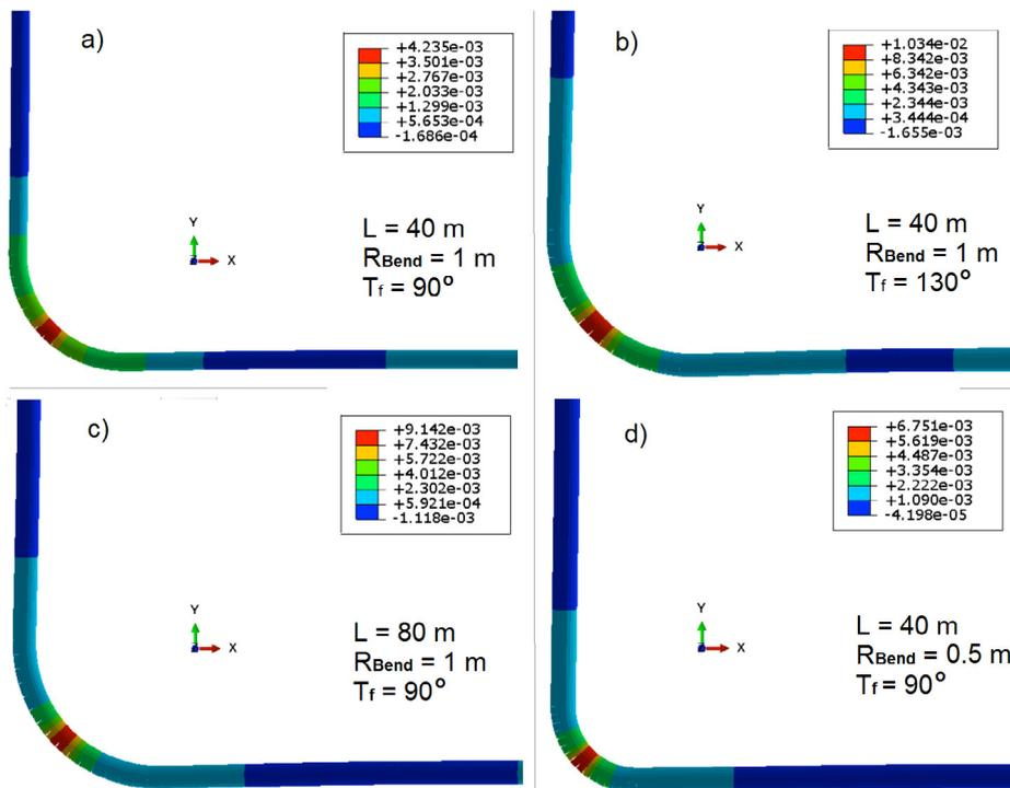
Fig. 2. Longitudinal strain contour and deformed shape of pipeline at the bend region, under operating conditions, for different values of the system parameters: a)  $T_f = 90^\circ\text{C}$ ,  $L = 40 \text{ m}$ ,  $R_{bend} = 1 \text{ m}$ ; b)  $T_f = 130^\circ\text{C}$ ,  $L = 40 \text{ m}$ ,  $R_{bend} = 1 \text{ m}$ ; c)  $T_f = 90^\circ\text{C}$ ,  $L = 80 \text{ m}$ ,  $R_{bend} = 1 \text{ m}$ ; d)  $T_f = 90^\circ\text{C}$ ,  $L = 40 \text{ m}$ ,  $R_{bend} = 0.5 \text{ m}$ .
