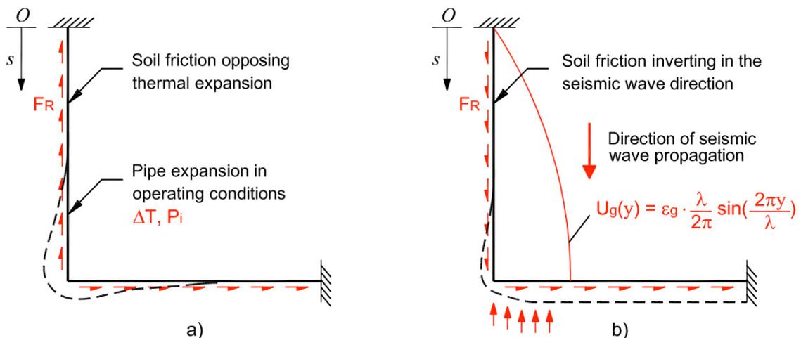
Fig. 7 Pipeline behaviour during: a) operating conditions; b) seismic ground deformation.
