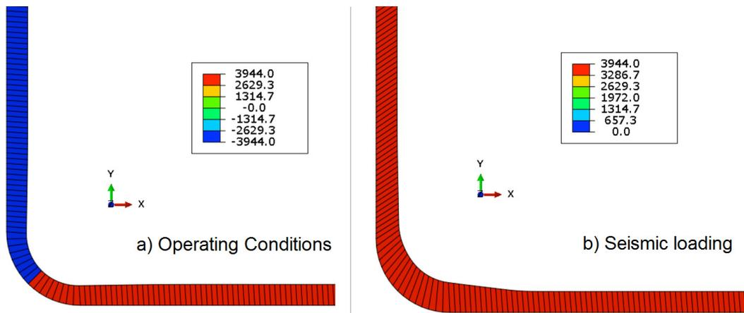
Fig. 5. Contour of the soil friction reaction along the pipeline (N/m): a) in operating conditions; b) under seismic loading.
