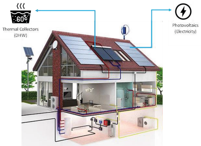
Figure 18 Recommended Solar Energy Mix of a Building Source: (CBSELECTRICS, 2014)
