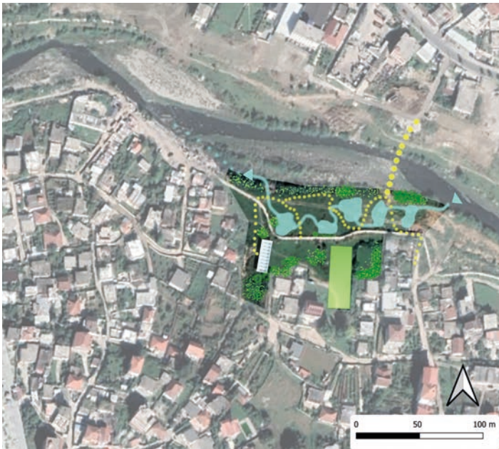
Figure 32 Concept Design of Filtration Ponds and Landscaping
