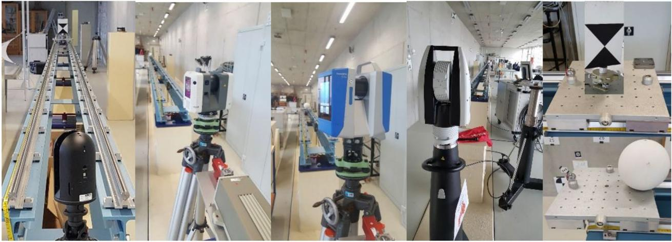
**Fig. 6** Terrestrial laser scanner at the comparator track (f.l.t.r.): Leica BLK360, Leica RTC360, Z+F IMAGER 5016, Leica Absolute Tracker AT960 (reference system 2017, 2020), and b/w target and sphere mounted on a metallic sledge
