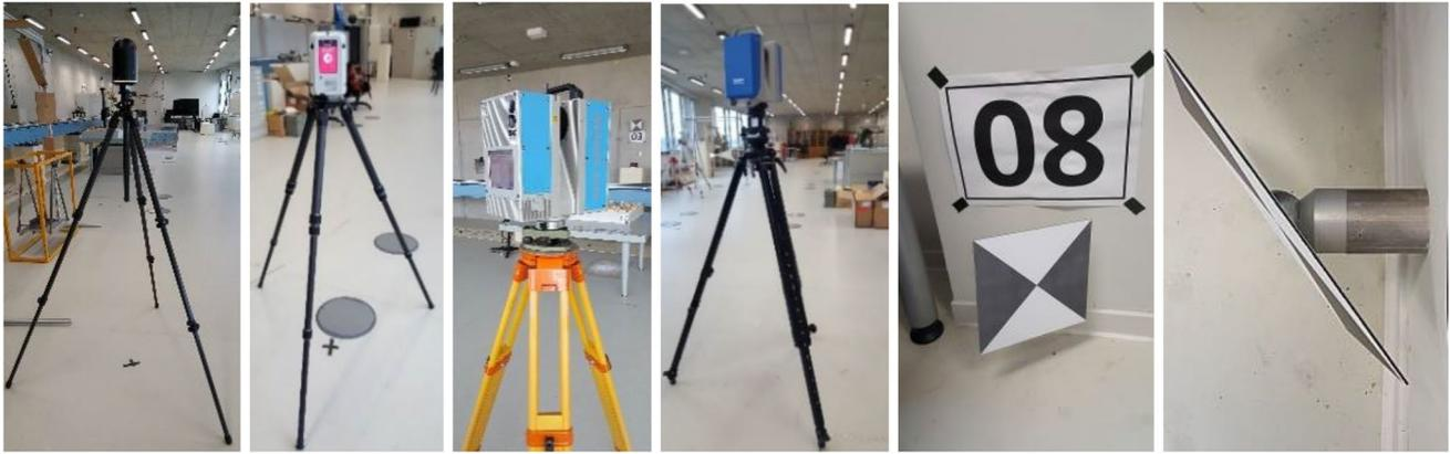
**Fig. 3** F.l.t.r.: terrestrial laser scanner Leica BLK360, Leica RTC360, Z+F IMAGER 5010, Z+F IMAGER 5016 in the 3D test field, and b/w target installation
