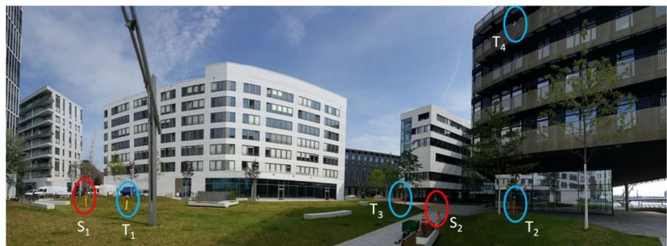
For the Faro scanner, all scans were performed as 360° scans with the scan parameter resolution 1/1 and quality 1× (which corresponds to 1.5 mm at 10-m distance and low measurement noise compression); each scan took approximately 15 min without colour acquisition.
