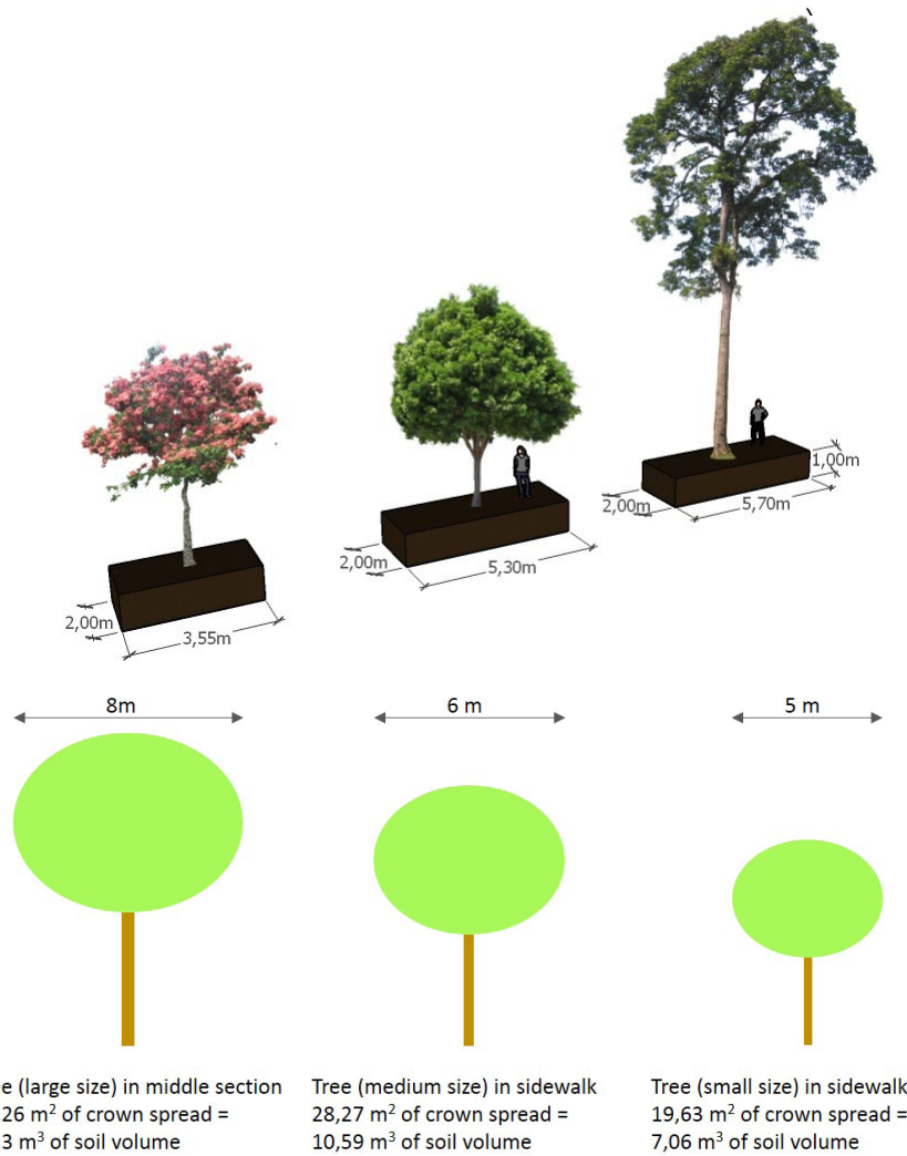
Figure 3:11 Soil volume requirements for selected tree sizes (author, 2015).
