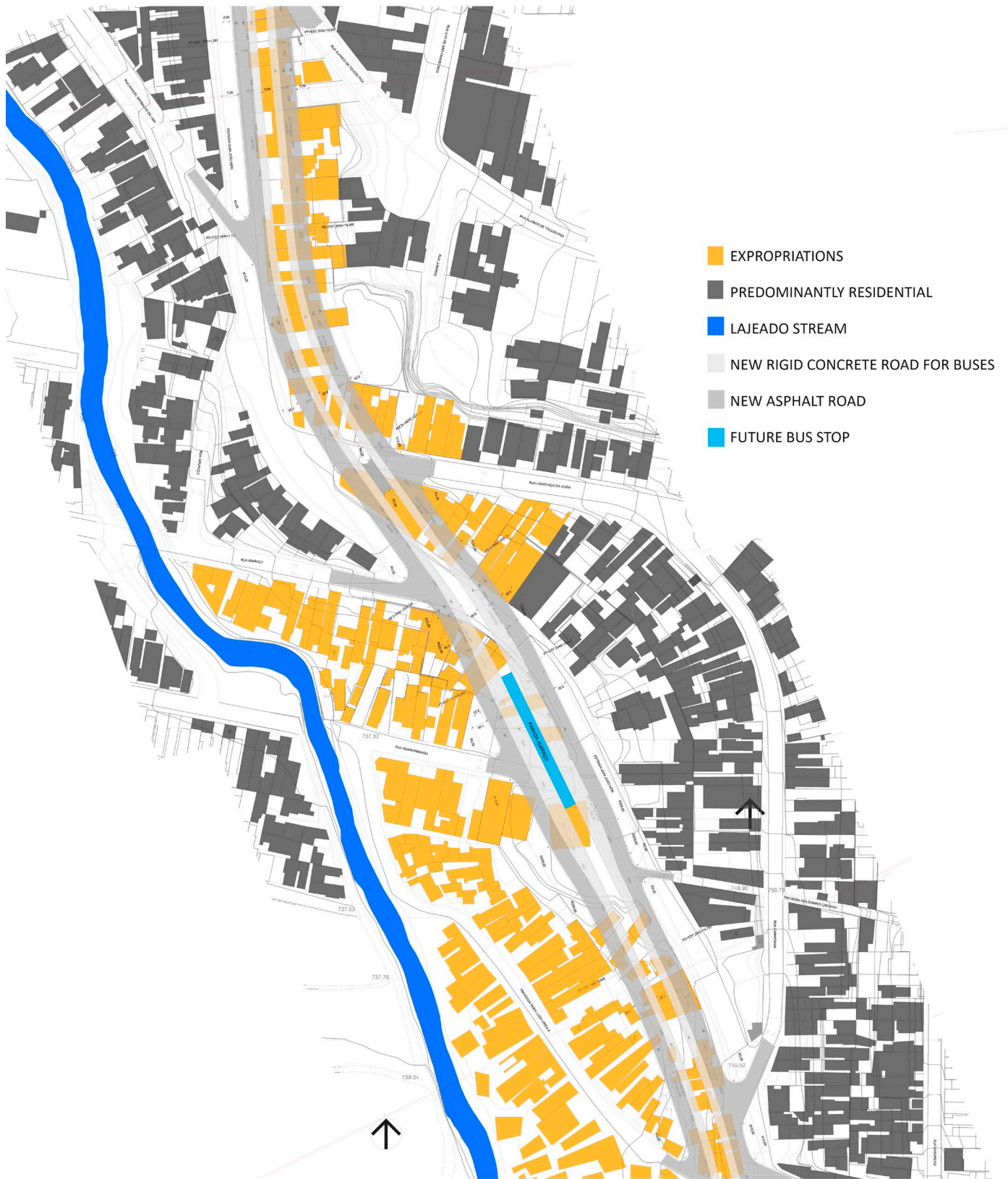
Figure 2:11 Plan showing the overlapping of proposed Itaim Paulista–São Mateus bus corridor with existing conditions (SPTrans, 2013; author, 2015).
