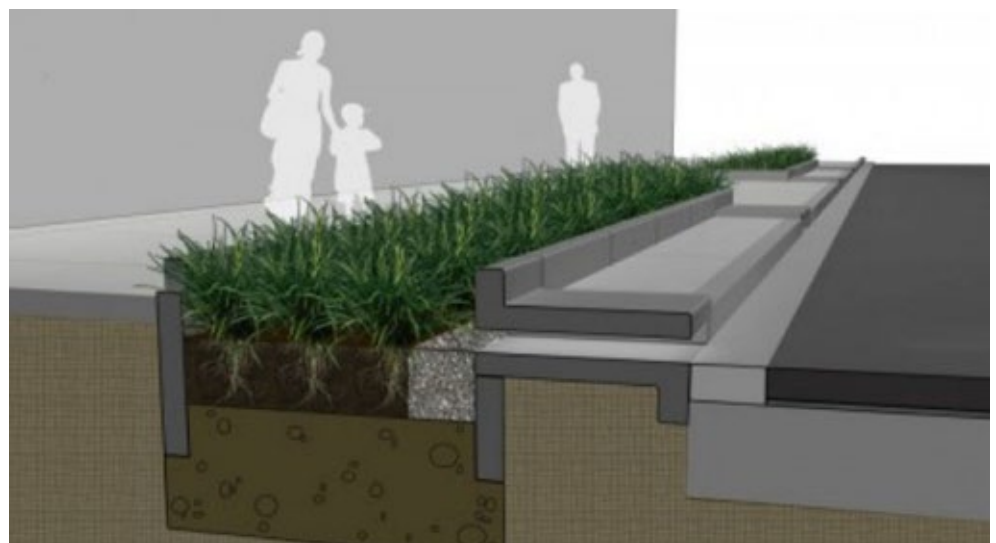
Figure 3:9 Diagrammatic section of a kerb-side rain garden system by HOK.
