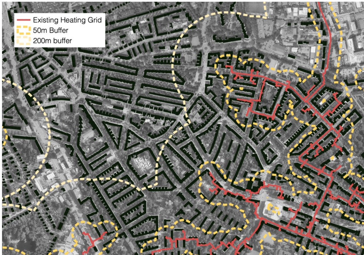
Figure 18. Different buffers (50 and 200m) around a district heating grid. Heating grids source: (Behörde für Umwelt und Energie [Hamburg Ministry for Environment and Energy], 2017), basemap source: (Freie und Hansestadt Hamburg, Landesbetrieb Geoinformation und Vermessung (LGV) [Hamburg State Office for Geoinformation and Surveying], 2022)
