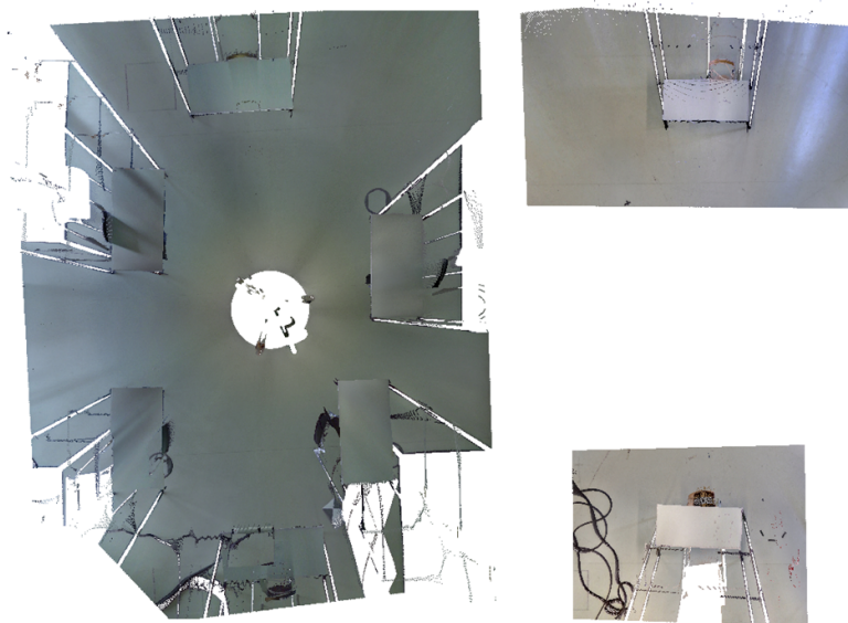
Figure 11. Points to be examined without semantic segmentation. Objects of the chair, table and floor classes, as well as scanning artifacts, are shown.
