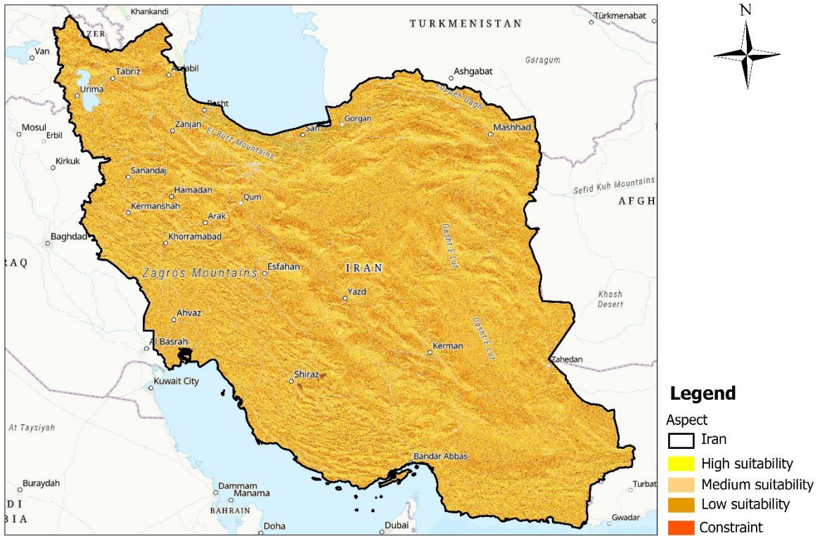
Figure 41 Assessment of land suitability for PV & CSP based on aspect criterion (by Author)
